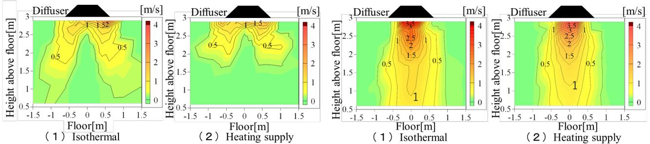
Figure 11. Wind speed of Y section(1/1 outlet)
