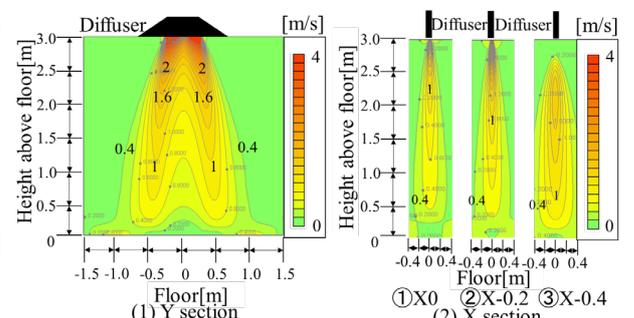
Figure 16. Wind speed of Y section(1/2 outlet) by CFD
