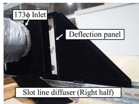
**Figure 2.** Photograph of the slot line diffuser
