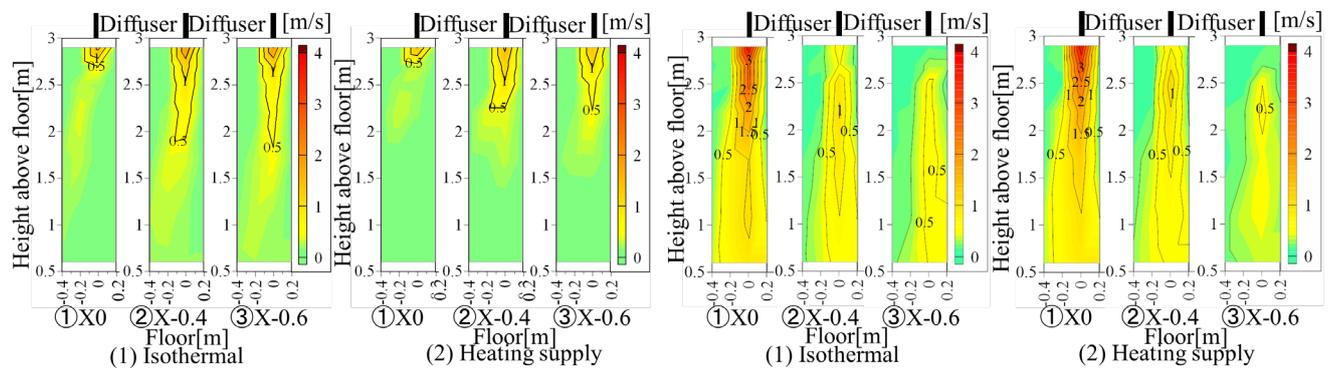
Figure 13. Wind speed of X section(1/1 outlet)
