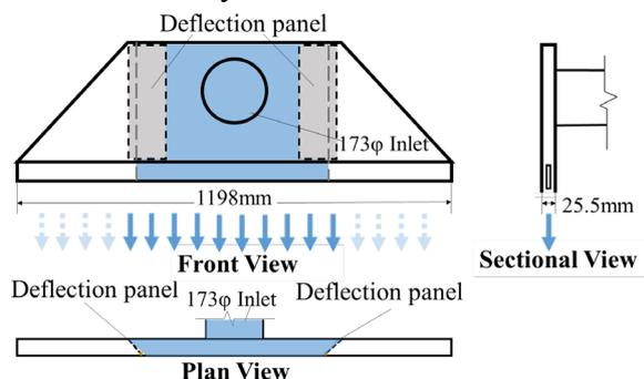
**Figure 1.** Detail view of the slot line diffuser
