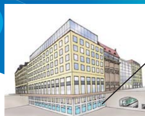
Building with Thermal Energy Storage (TES) Tank
