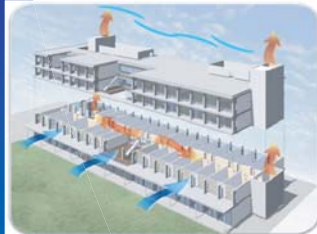
Natural Ventilation System through Staircase Chimney
