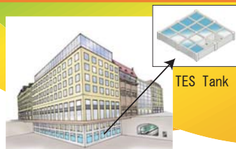
Building with Thermal Energy Storage (TES) Tank
