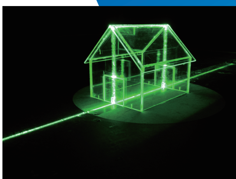
Wind Tunnel Test for Detached House
